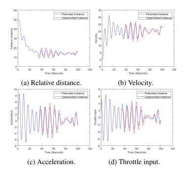
Figure 3: The propagation of an error in the vehicle features of follower vehicle 1 due to a perturbation.
