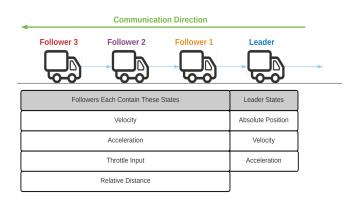
Figure 2: Vehicle features of 1D platooning model from [15].
